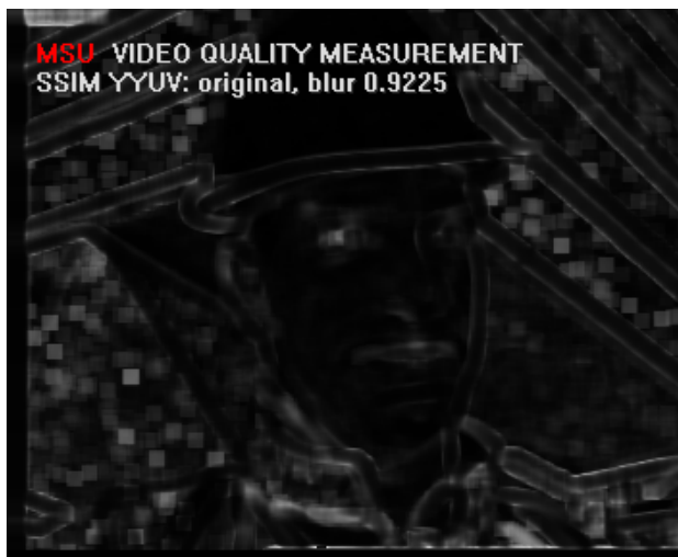
(c) SSIM map for blurred image, SSIM = 0.9225
